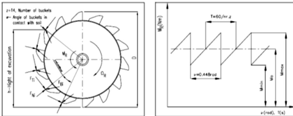
Fig. 4. Forces acting on bucket wheel and saw like load due to bucket spacing
