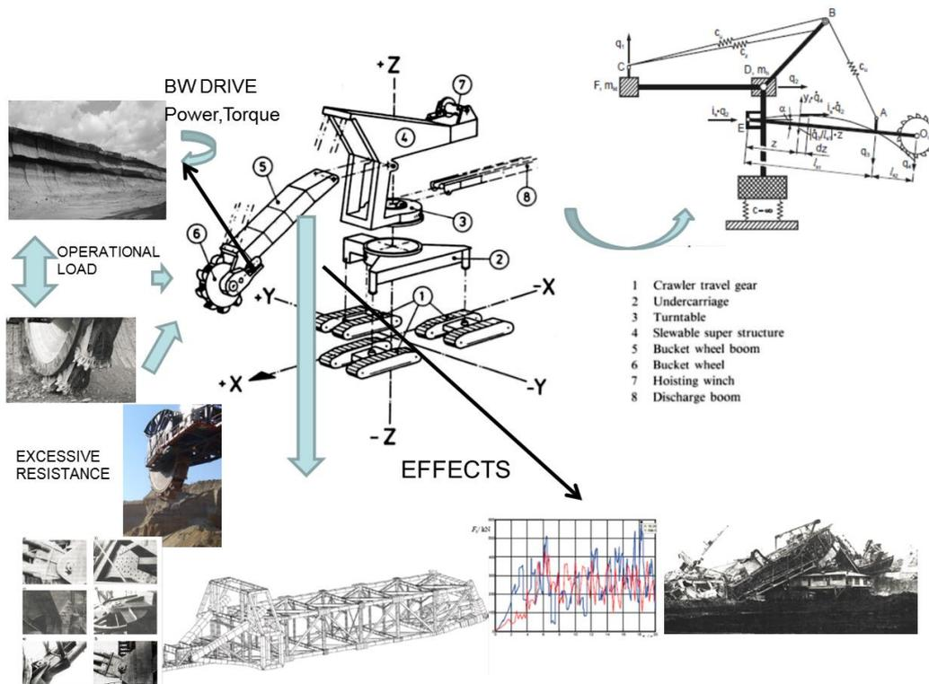
Fig. 1. Logic scheme of the complex problem of excavating hard formations/inclusions with BWE
