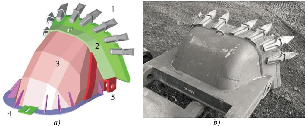
**Fig. 6.** Typical bucket design 1 Tooth, 2 Lip, 3 shell, 4 attachments a) rounded b) rectangular
