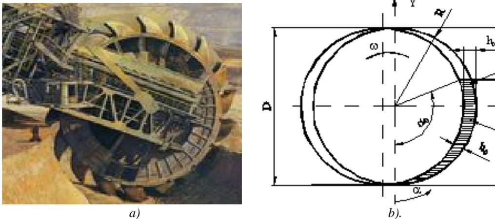
Fig. 5. Typical bucket wheel (a) cutting height relative to BW diameter (b)
