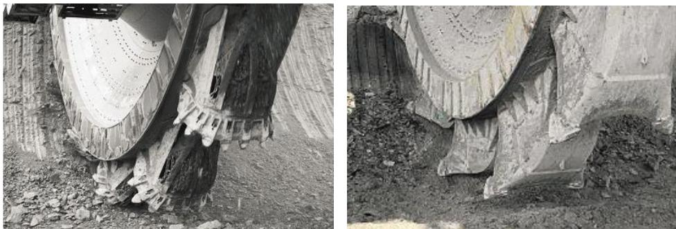
**Fig. 7.** a) Chain mat instead of shell of buckets b) bucket with corner cutters for soft material
